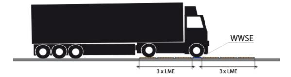
NOTES: The best weighing condition is obtained by creating a levelling area of a length equal to double that of the longest vehicle to be weighed.
